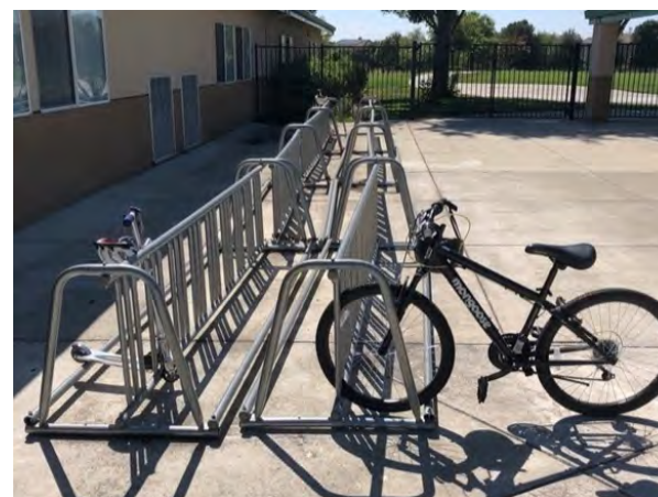
The bike racks are currently pushed against each other, reducing parking capacity by half.
