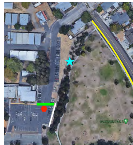
The recommended improvements for an alternate drop-off area prioritize reducing interactions between motorists and student pedestrians and bicyclists. The yellow represents the new drop-off zone, the blue star marks the location of a culvert bridge, the white line represents the extension of the Community Park 2 path, the green line represents the raised crosswalk, and the red hexagon marks the location of a new crossing guard.
