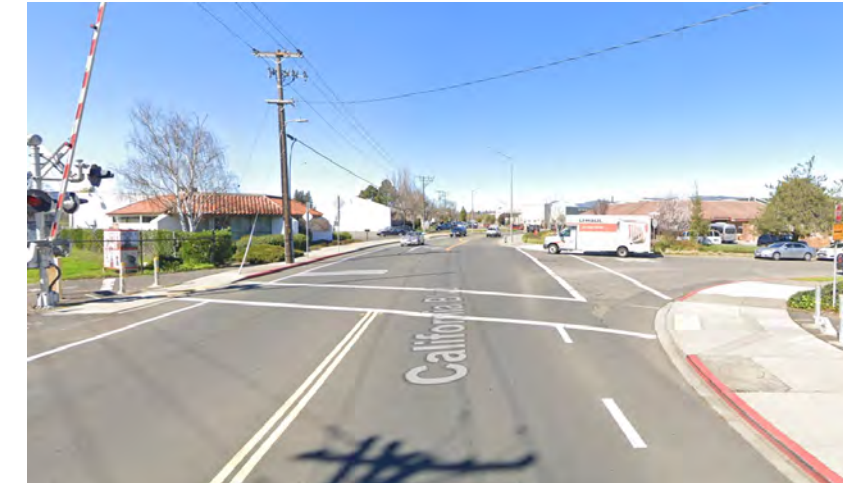
Long crossing distances and uncontrolled traffic on California Boulevard make the intersection challenging for bicyclists and pedestrians.
